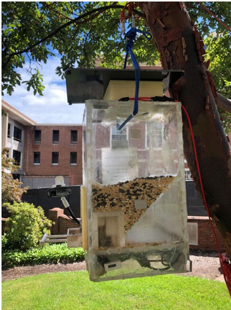
FIGURE A2 A side view of our PASSER smart feeder at the campus location
